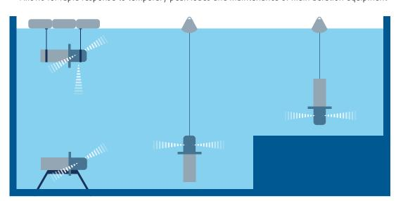
Flexible installation. Submerged venturi mixer for better mixing power and improved dissolved oxygen distribution. Nozzles can be blocked to enable horizontal mounting.
