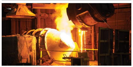
Invented in 1954, Linde's proprietary argon oxygen decarburization (AOD) process was first used exclusively for stainless steel production; now it is used to produce military grade steels, tool steels, carbon and low-alloy steels, nickel grades, cobalt grades, and superalloys.
