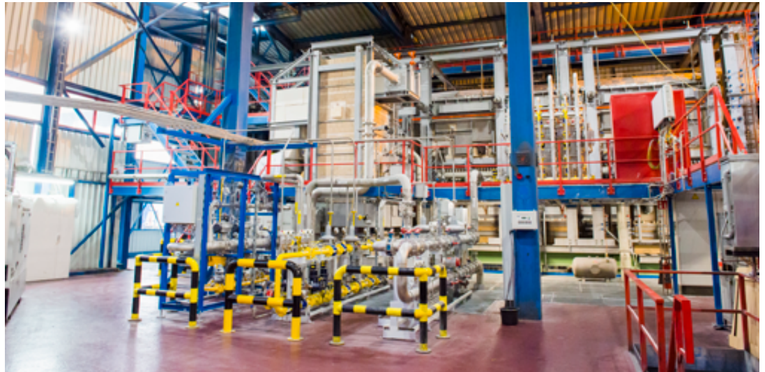
Linde's OPTIMELT™ ThermoChemical Regenerator Can Reduce Fuel Consumption Up To 30% Compared To Air-Fuel Glass Furnaces.
