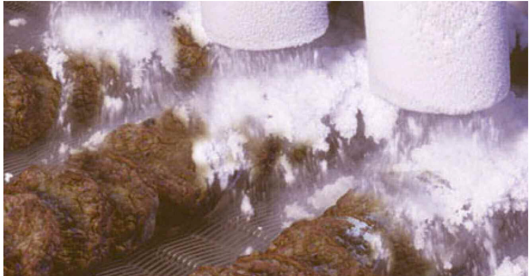
Carbon dioxide snow can be directly applied with the exact volume and pattern required for in-line chilling purposes
