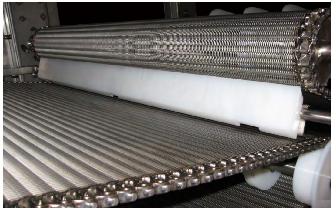
Close up of a cascading belt flight and nylon guide bar.
