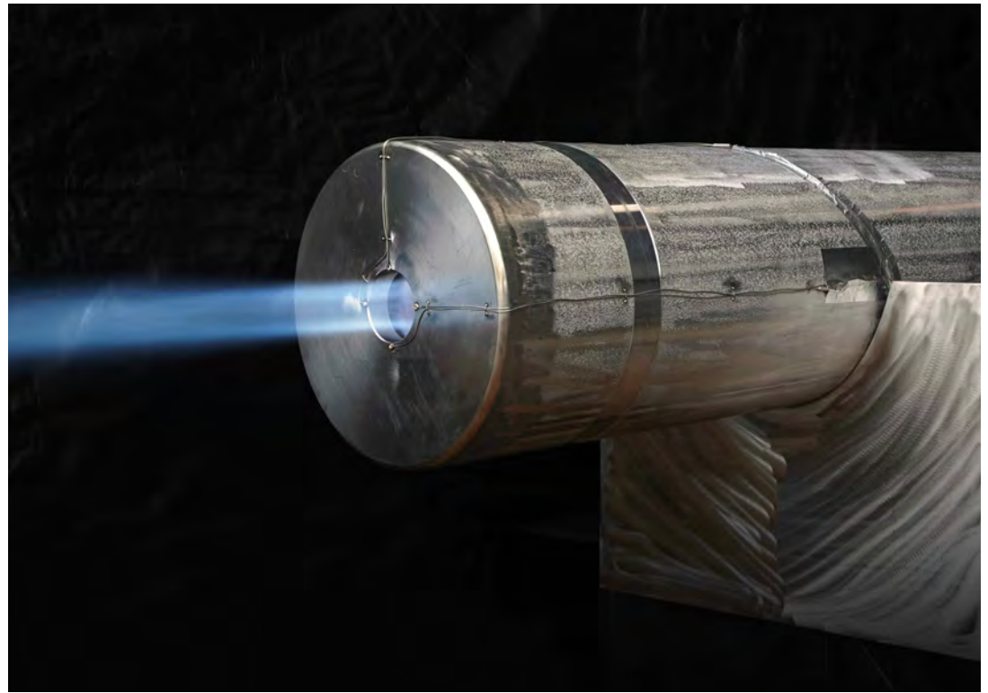
The commercial scale Hot Oxygen Burner (HOB) shown is capable of heating 300 tons per day of oxygen. The HOB system was designed for reforming syngas (99.9% tar and hydrocarbon conversion) produced from gasification of municipal waste. The same design can be used to reform syngas from various biomass and hydrocarbon feedstocks and fuel. Heating the oxygen can be provided by natural gas, propane or recycled tail gas from downstream processes.
