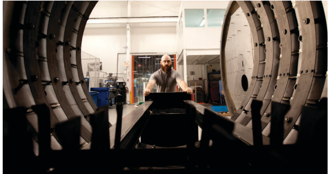
Industrial autoclaves pressurized with nitrogen assist in heat transfer and provide a safer inert atmosphere.
