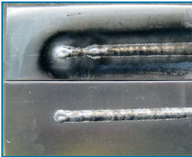
Fig. 2 Weld of Aluminium before and after "Cryoclean" snow treatment.
