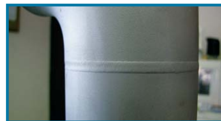
Fig. 5. "CryoAdd" removes oxides from orbital welds.
