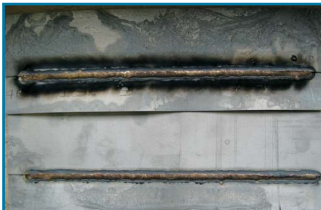
Fig. 3 Soldered zinc-plated sheets before and after "Cryoclean" snow treatment.
